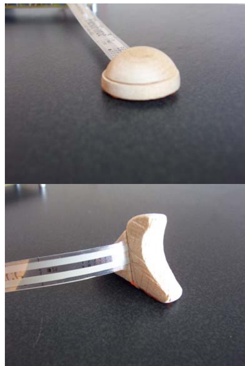
Figure 3: Force sensing resistors embedded into wooden hemisphere and trigger.
