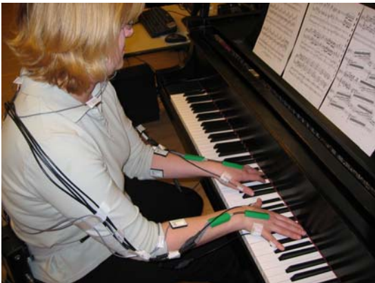
Figure 2. Subject wearing electrogoniometers and sEMG instrumentation while performing the excerpt
